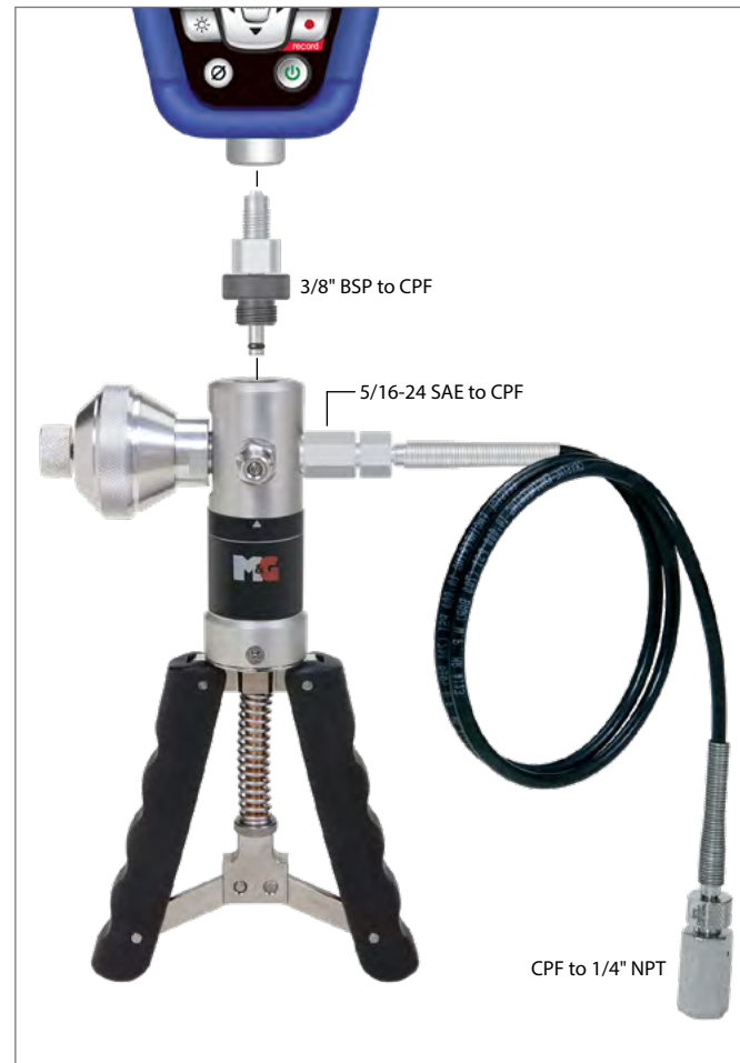
Crystal CPF fitting connection.
