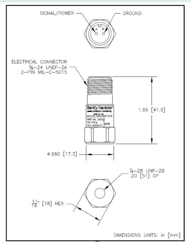
Figure 3: 200350 Accelerometer Sensor
