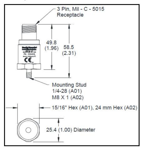
Figure 5: 330400/330425 Accelerometer Sensor
