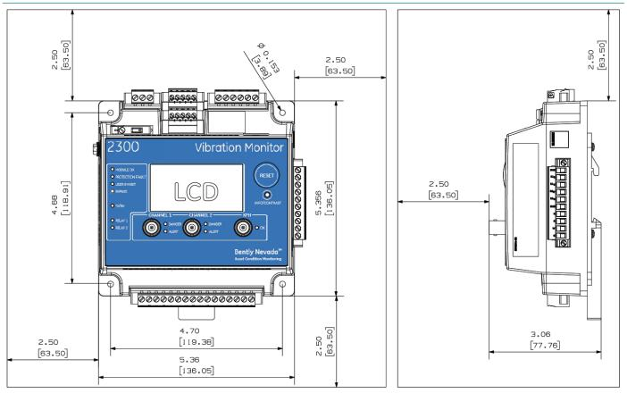
Figure 12: 2300 Series Monitor Recommended Clearance
