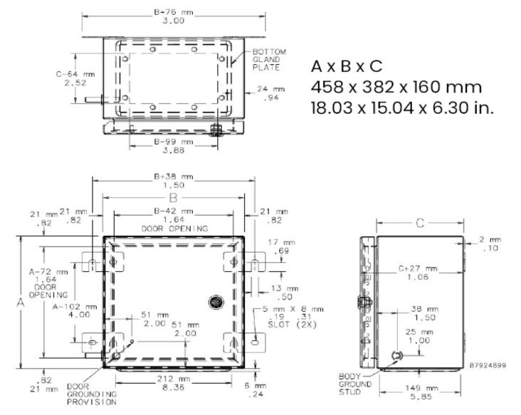
Figure 1: 105M6193-03 Weatherproof Housing
