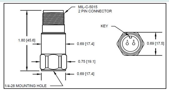
Figure 4: AM3100T2-Z2 Accelerometer Sensor
