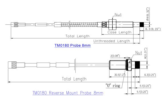
(Works with TM0181 cables and TM0182 drivers)
